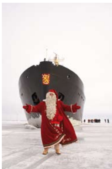
Icebreaker Sampo can take 150 passengers on board. There are sixteen people in the crew. The length of the vessel is 75 meters, beam 17,5 meters and draught 7 meters. The 4 main engines can generate 8 800 horse powers.
